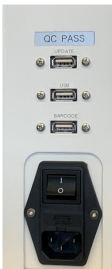
Figure 19. Data Update, USB and Barcode reader port location at the back of the machine.
