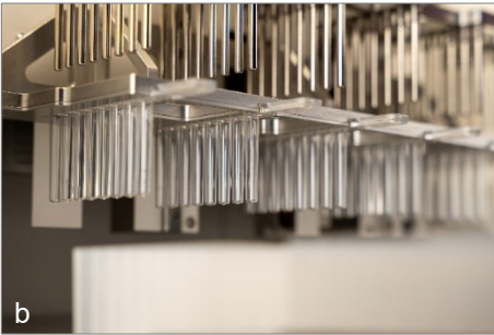
Figure 9. Rod covers (a) and their dedicated positions in the instrument (b).
