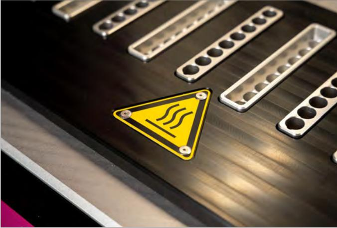
Figura 6. Heating block (Bloque calefactor).
