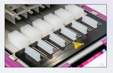
Lysis occurs in the lysis strip. Up to 3 wash steps and elution are performed in the 32-well block. Heating and/or cooling of lysis is optional.
