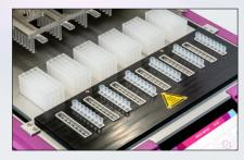
Lysis and up to 3 wash steps occur in the 32-well block. Elution occurs in the elution strip. Heating and/or cooling of elution is optional.
