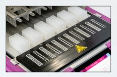
All extraction steps are performed in the 32-well block – lysis, up to 2 wash steps, and elution - with no heating or cooling.
