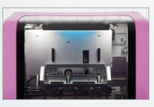
Integrated UV light with an adjustable timer ensures process safety and covers the entire deck.
